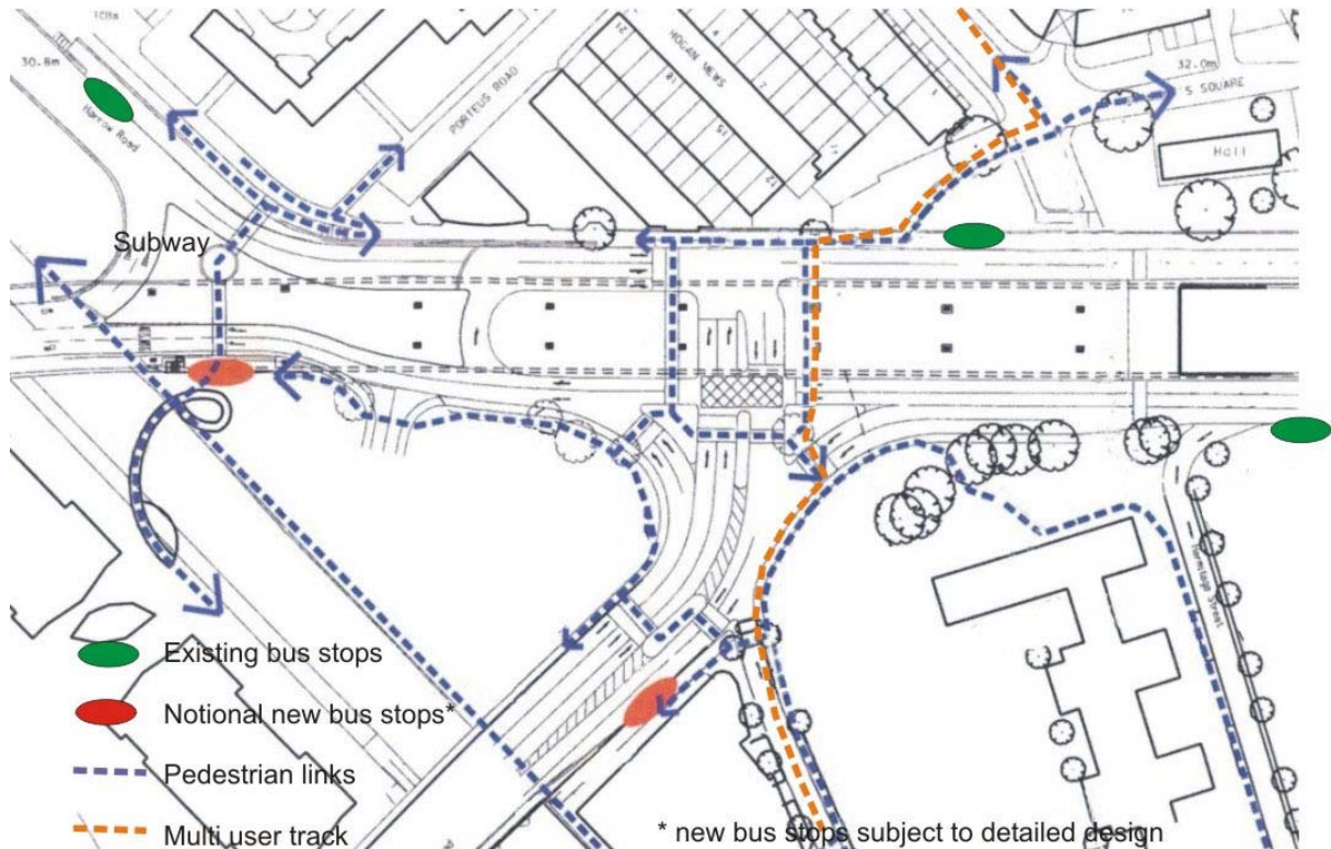
The simplified junction that is basically a signalised "T" junction and indicative pedestrian routes.
