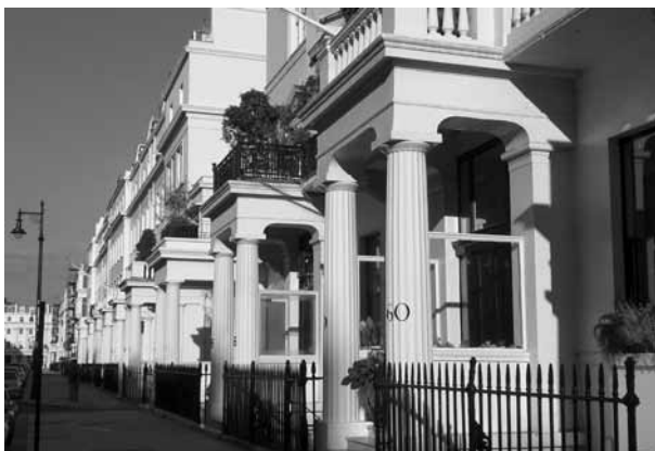
Figure 31: Repeated detail of projecting fluted Doric porticos creates rhythm and uniformity in the street scene.
