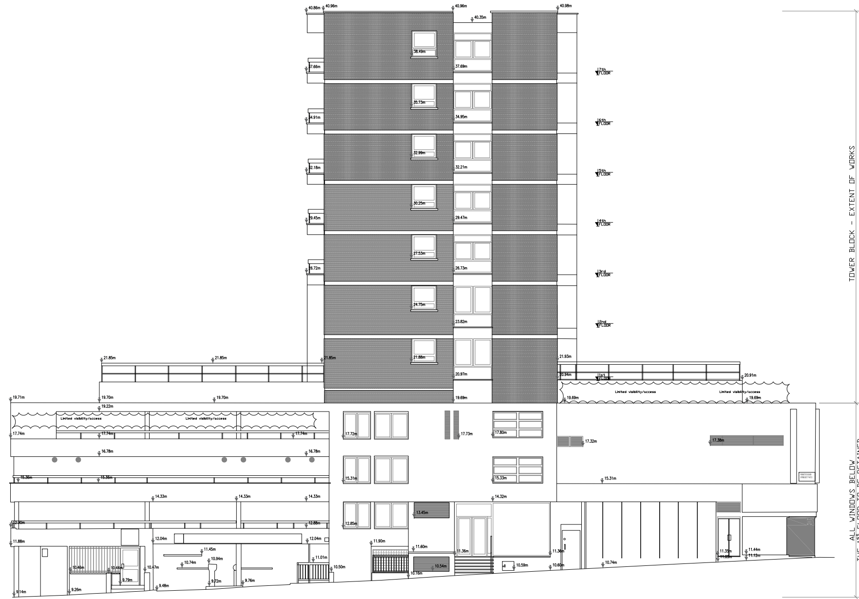
EAST ELEVATION AS EXISTING (SCALE 1:100@A1; 1:200@A3)
