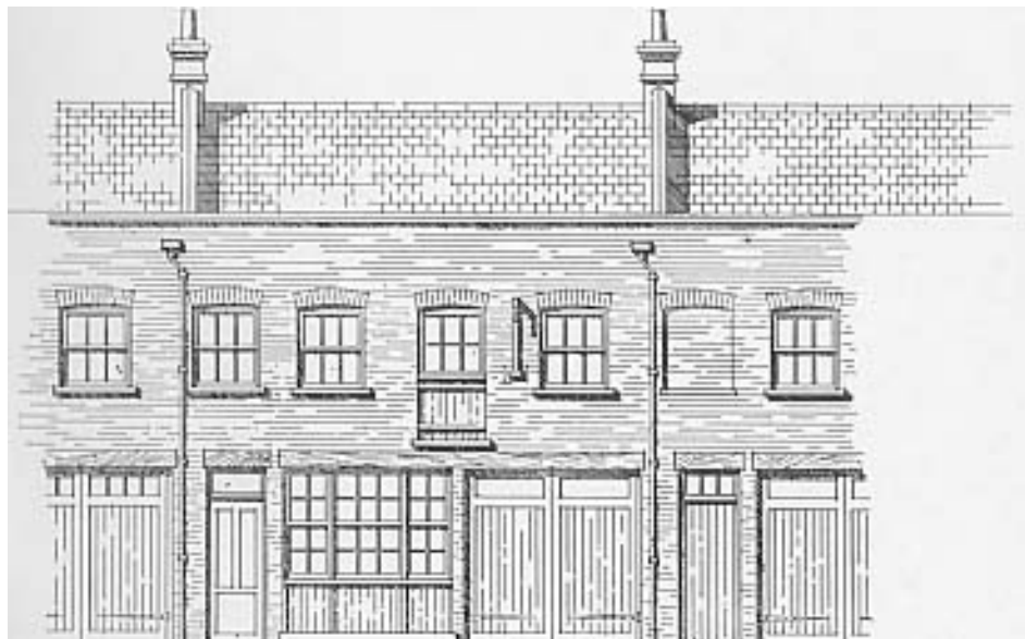
Fig. 1A: Possible Alterations to Front Elevation for the Conversion of a Mews-building to a House, without a Roof Extension. The Council will encourage conversions which retain the form of the original roof, subject to local considerations in individual cases.
