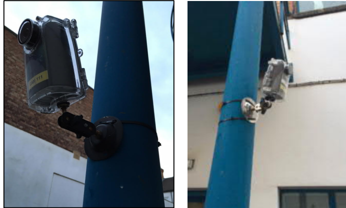
Example of small monitoring cameras with suitable housings and mounting
