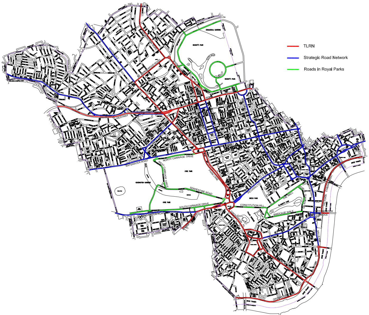
Figure 1: Map showing the inter-relationship of Transport for London Road Network (TLRN) [Red], Strategic Road Network (SRN) [Blue] and Roads in Royal Parks (Green)
