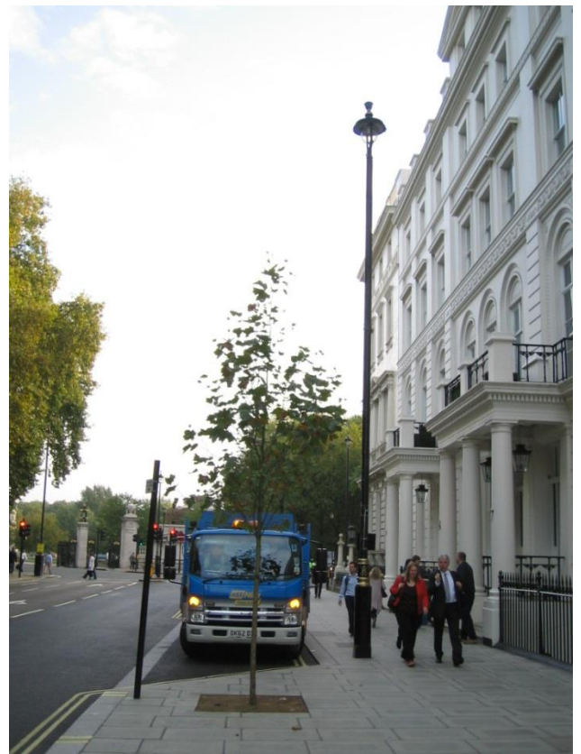
Trees planted 'in front' of line of columns which as they mature will block the performance of the lighting
