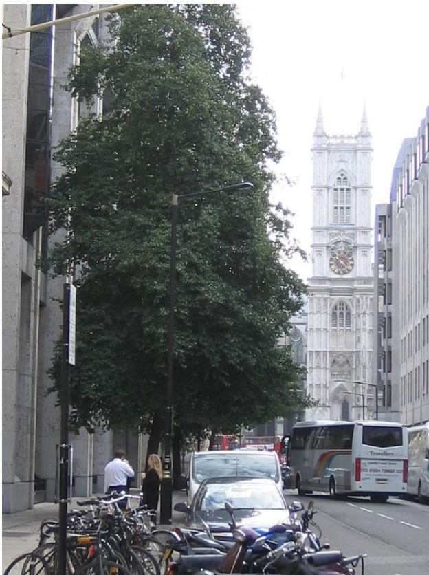
Lighting column with bracket adjacent to tree, the canopy having grown out across the street thus blocking off light to the footway and road past the tree.
