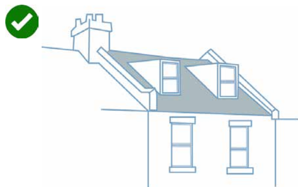
Figure 69: Diagram showing 2 small dormers in line with the windows on the storey below
