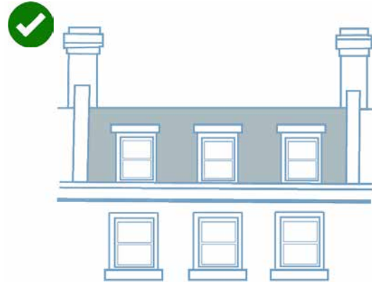
Figure 71: Diagram of a well designed flat mansard roof extension. Based on Westminster 'A Guide to Alterations and Extensions on Domestic Buildings SPD'
