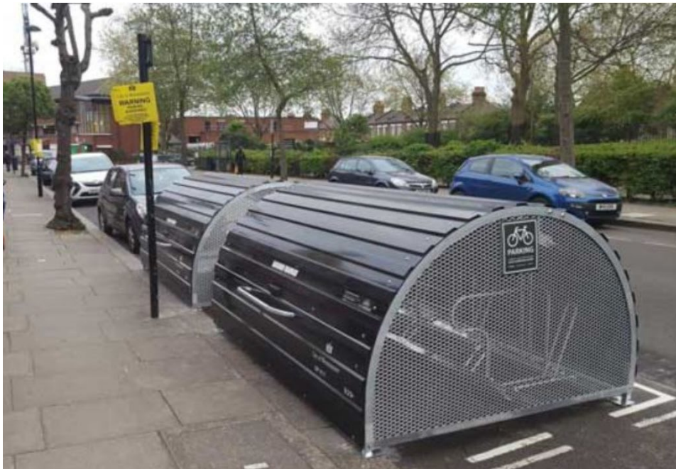
Figure 30: Cycle hangar in repurposed half a car parking space, with space for 6 bikes, with covered weather protection. They are approximately 2.6m wide, 1.3m high (Open: 2.3m), 2.0m deep and painted black to match existing street furniture in Westminster.
